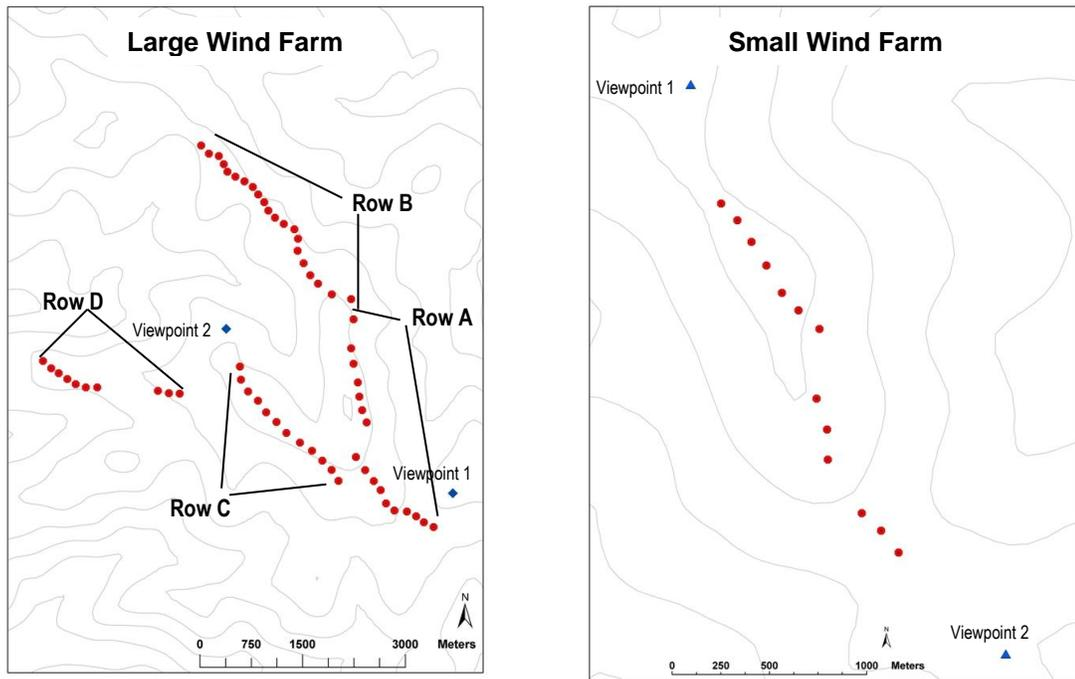
**Figure 2.** Distribution of the turbines in the two wind farms monitored in 2004.
